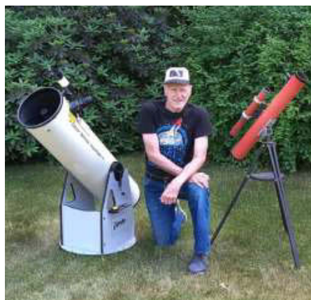
▲ The author poses with the two telescopes through which he's seen a large number of asteroids. The red telescope is Edmund Scientific's Space Conqueror, a 3-inch f/10 reflector. The larger scope is a 10-inch f/5 reflector. GLENN CHAPLE
